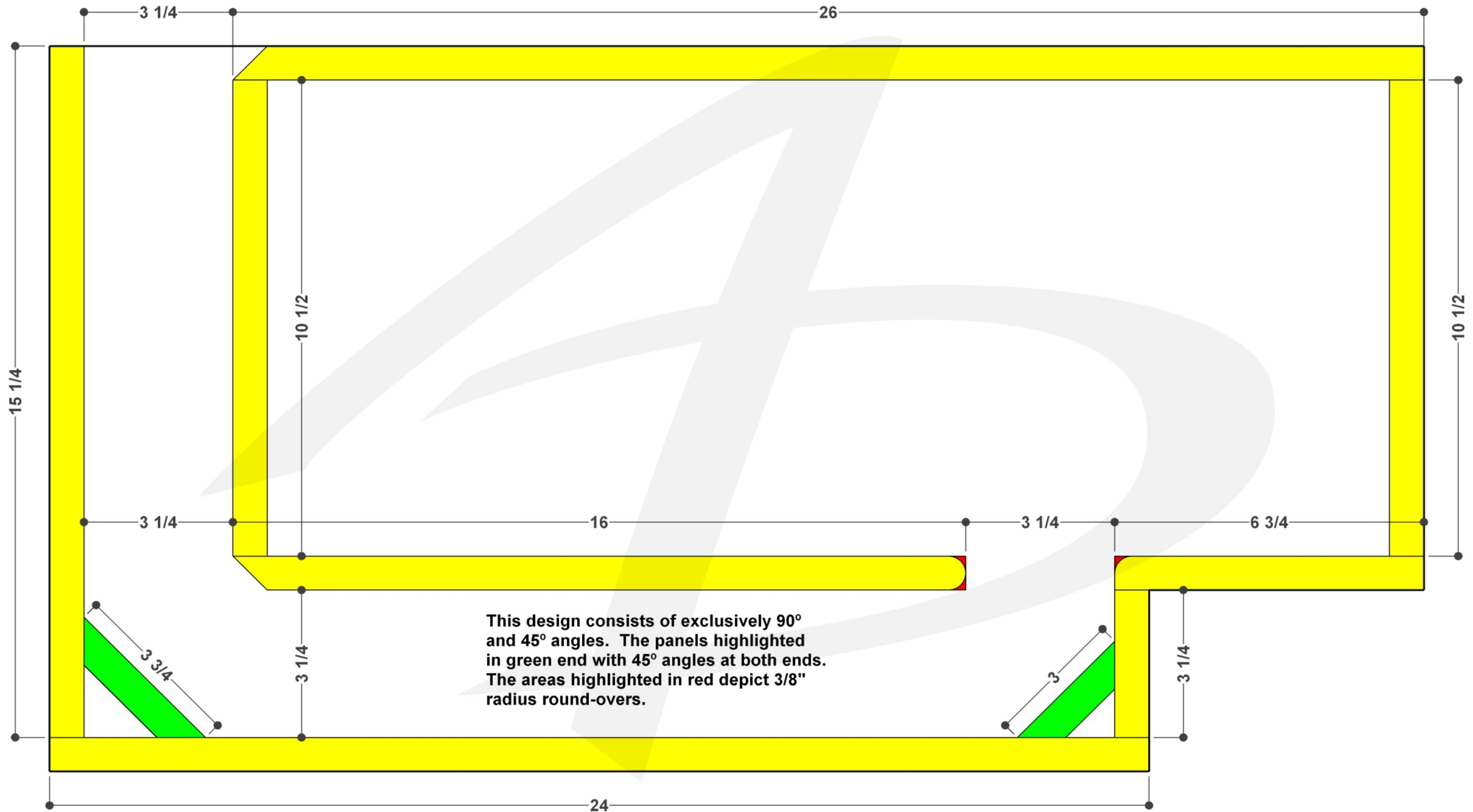
This design consists of exclusively 90° and 45° angles. The panels highlighted in green end with 45° angles at both ends. The areas highlighted in red depict 3/8" radius round-overs.
